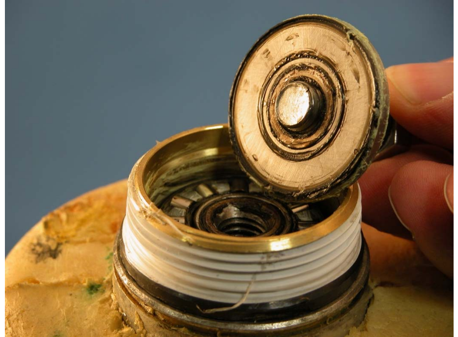
Unscrew Bolt, Remove Thrust Washer
